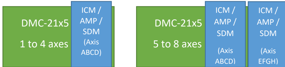
1-4 axis DMC-21x5 model (left); 5-8 axis DMC-21x5 model (right). An ICM is selected when internal amplifier is not required on a group of 4-axis.
